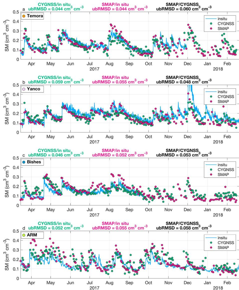
**Figure 5.** In situ soil moisture observations from four COSMOS sites (indicated by the colored dots shown on the map in Figure 4c), Soil Moisture Active Passive (SMAP) soil moisture (SM) retrievals, and Cyclone Global Navigation Satellite System (CYGNSS)-derived SM for the same locations. ubRMSD = unbiased root-mean-square difference.
