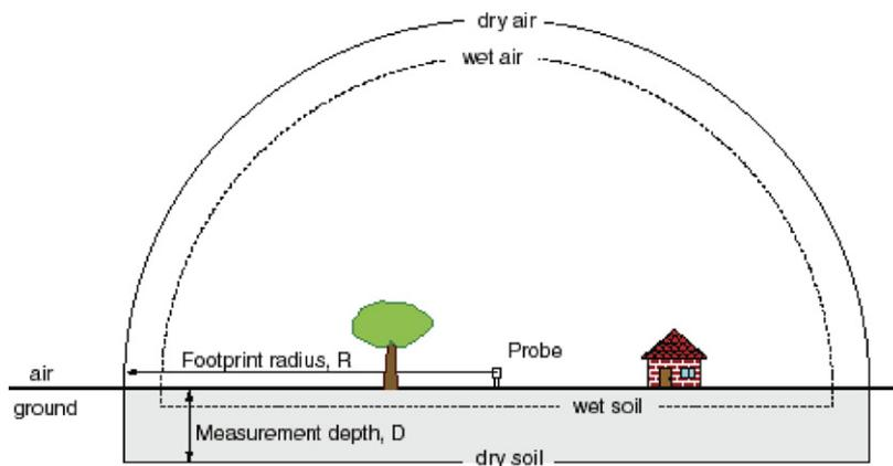
**Fig. 2.** Sensing volume of the cosmic-ray probe comprises a hemisphere in air (of radius  $R$ ) and a cylinder in soil (of height  $D$ ). All hydrogen within the sensing volume is reflected in the measured neutron intensity. The horizontal footprint,  $R$ , depends on air properties: mainly density and water vapor content. The vertical footprint depends on soil properties: mainly bulk density and total hydrogen content (pore water, lattice water, and organic matter water).
