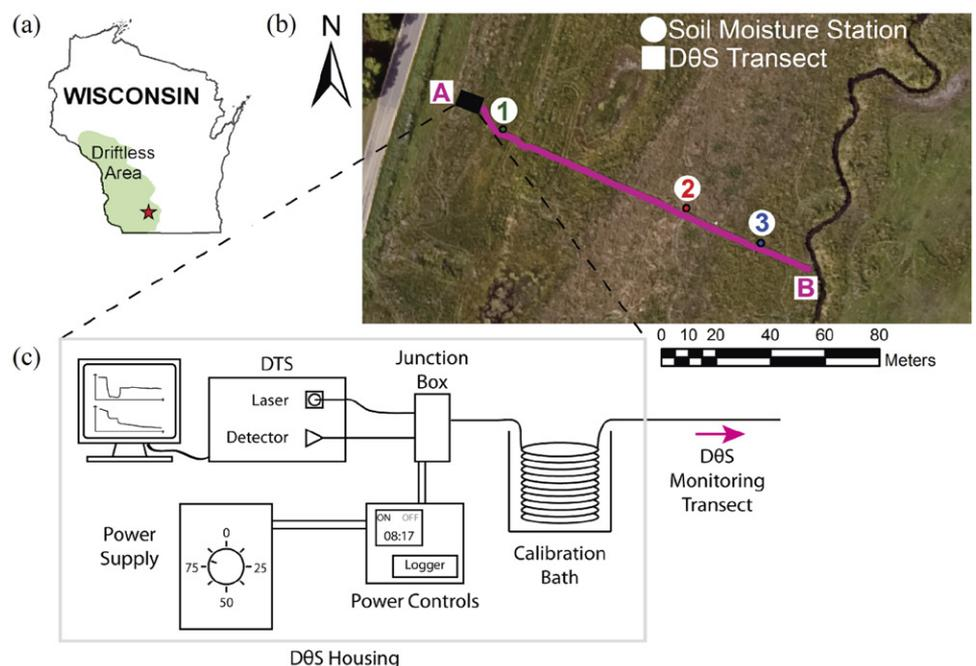
**Fig. 5.** (a) Location of study site used by Striegl and Loheide (2012), (b) aerial photo of active distributed temperature sensing (DTS/DθS) transect with three independent soil moisture ( $\theta$ ) monitoring stations, and (c) schematic diagram of active DTS system components (Reprinted from *Groundwater* with permission of the National Ground Water Association. Copyright 2012; Striegl and Loheide, 2012).
