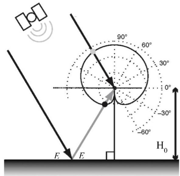
**Fig. 3.** Geometry of a multipath signal, for antenna height ( $H_0$ ) and satellite elevation angle ( $E$ ). Black arrows represent the direct signal transmitted from the satellite. The gray arrow is the reflected signal from the ground. The solid line represents the gain pattern of the antenna. Dashed circles indicate relative power levels of the gain pattern (Reprinted from Larson et al., 2008a with permission from Springer-Verlag.).
