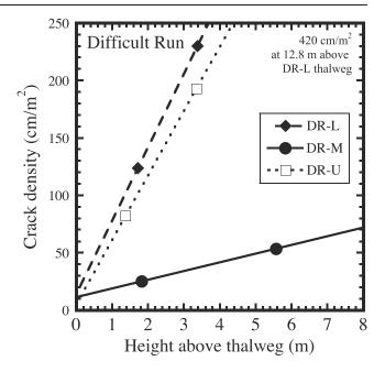
**Figure 8.** Comparison of crack density with height above the thalweg on Difficult Run (DR). Text in upper right corner reports the crack density measured at an outcrop on the adjacent hillslope. Though our data is limited, we see an increase in crack density with height above the thalweg in all three cross-sections (DR-U, DR-M, DR-L).
