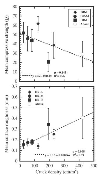
**Figure 10.** Comparison between crack density and mean rock compressive strength (top) and crack density and mean surface roughness (bottom). In general, compressive strength decreases and surface roughness increases as crack density increases. Error bars represent one standard deviation. We find a significant linear relationship between crack density and surface roughness ( $\rho$  = 0.008), but not for crack density and compressive strength ( $\rho$  = 0.145).
