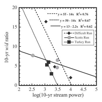
**Figure 11.** Relationships between stream power (surrogate for cross-section average erosion rate) and channel cross-section width/depth (w/d) ratio, both calculated for the estimated 10-year flow. In all three channels, the w/d ratio becomes smaller at higher values of stream power. However, the number of cross-sections measured is too low to draw statistically significant conclusions.
