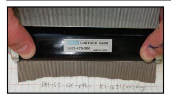
**Figure 4.** Contour gage photographed after being pressed perpendicularly against the bedrock surface. Photographs were processed using image analysis to determine surface roughness, calculated as the standard deviation of pin heights. [Colour figure can be viewed at wileyonlinelibrary.com]
