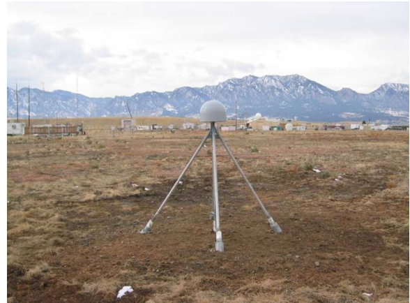
Fig. 1. Continuously operating geodetic quality GPS receiver operating as part of the Earthscope Plate Boundary Observatory. This site in Marshall, CO, was used for the GPS soil moisture calibration study.
