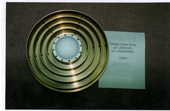
Fig. 3. Top view of the antenna used by the Plate Boundary Observatory and many other geodetic-quality GPS receivers.
